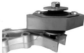
Run the car for a about 5 miles. If the vibration feels excessive slacken the two 8mm screws and the same screws on the gearbox side mount and physically rock the engine back and forward by hand then retighten all screws. This should allow the engine to centralise in a neutral load position.
